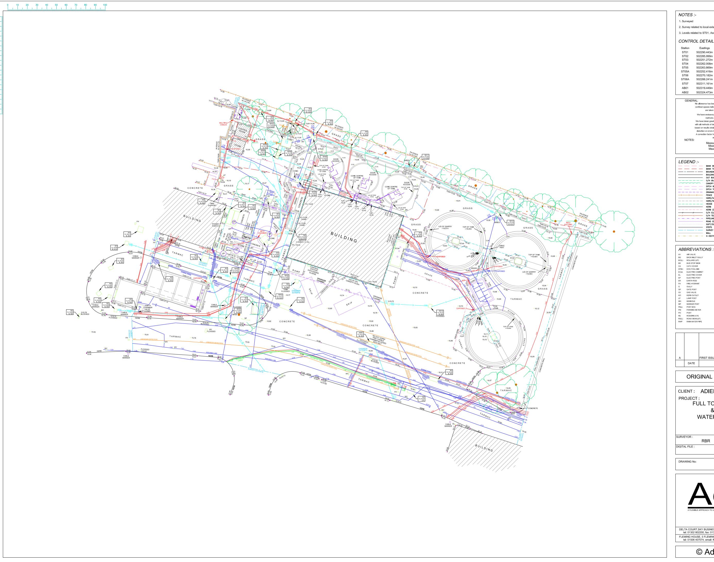
NOTES :-1. Surveyed 2. Survey related to local existing metric grid. 3. Levels related to ST01. Assumed value = 15.987m CONTROL DETAILS :-Elevation ST01 502290.443m 171749.458m 15.987m ST02 502285.999m 171766.866m 15.961m ST03 502251.272m 171750.438m 15.922m Nail 171779.461m ST04 502262.008m 16.055m ST05 502263.869m 171787.780m 16.081m ST05A 502252.416m 171788.140m
